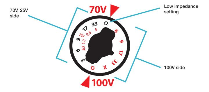
**Low impedance/transformer-bypass mode:** Match up the  $\Omega$  symbol to both arrows (like shown above).
