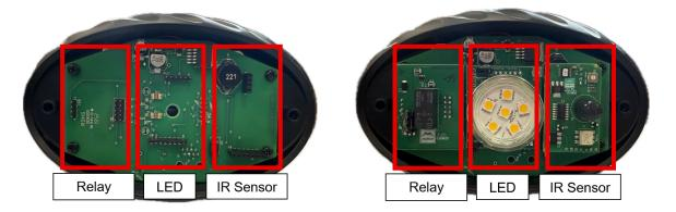
Install the FP-LIGHT MODULE Lamp Baffle/Lens and/or FP-MOTION MODULE
