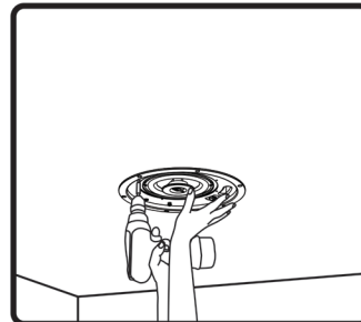
7. Insert speaker into mounting hole. Screw down both bolts on the baffle face to actuate the mounting wings. Firmly secure both bolts – do not over-tighten.
